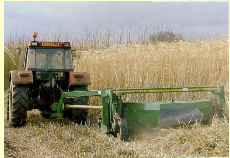
Figure 4.5 Harvesting miscanthus using conventional agricultural machinery
